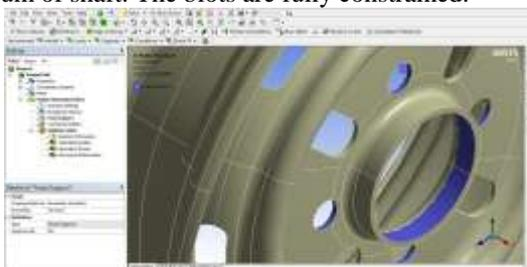
Figure 6 : Constraints on a car rim
