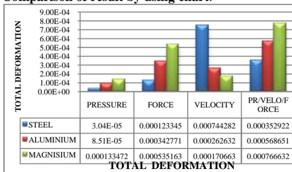
Graph : Variation in Total Deformation due to change of boundary condition and Materials.
