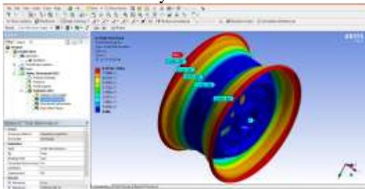
Figure 14:-Total Deformation (Al)
