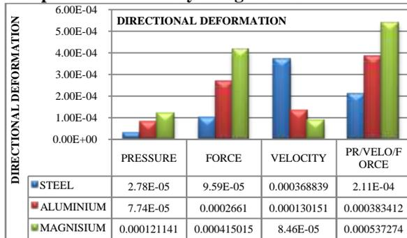
Graph : Variation in Directional Deformation due to change of boundary condition and Materials.
